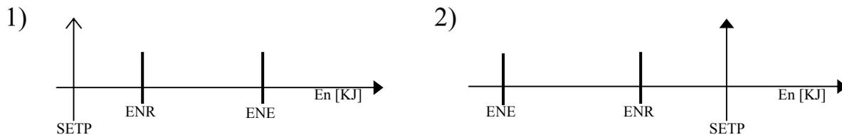
In both the conditions described above in the graphs (1, 2), it is not useful to open the outside damper as the inside enthalpy is closer than the outside enthalpy to the enthalpy set point.
