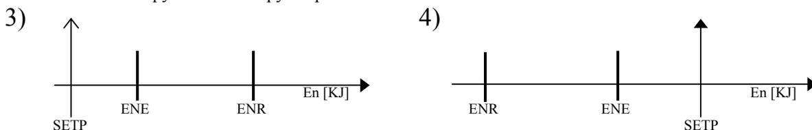
In both the conditions described above in the graphs (3, 4), it is useful to open the damper as the outside enthalpy is closer than the inside enthalpy to the enthalpy set point.
