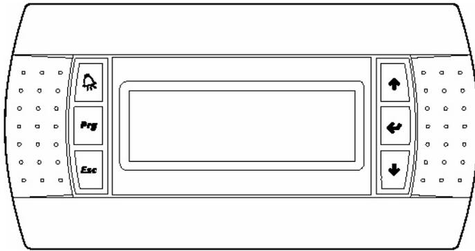
The operation of the PGD0 terminal is very similar to the Built-In terminal (access to the loop of screens, on/off, etc.) To switch between boards using a shared terminal PGD, access screen M2 by pressing the **UP** or **DOWN** buttons on screen M0 (main screen).
